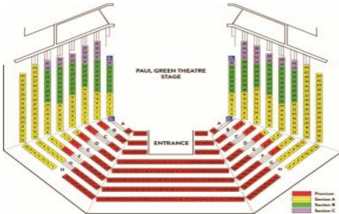
Figure 1. Paul Green Theatre seating chart, a “Thrust” design auditorium Within our sample we observed that unless the auditorium is a ‘thrust’ design (such as a Paul Green Theatre - see Figure 1), there is a very precise linear correlation between the root of seating capacity and the number of rows, just as we had hoped.
